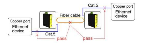
Both Ethernet devices will also detect a link fault on each Cat.5 connection, although the real fault occurs on the fiber connection exactly.
