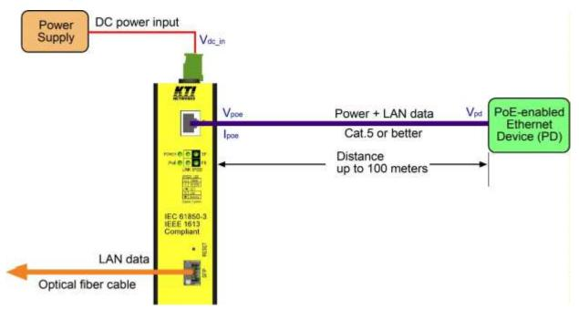
The device is equipped with PoE PSE function, which can supply power to a remote Ethernet device together with LAN data via TP port over Cat.5 cable. Above figure is a standard PoE connection example. By auto-detection and classification, the device supports the following PD types and classes:
