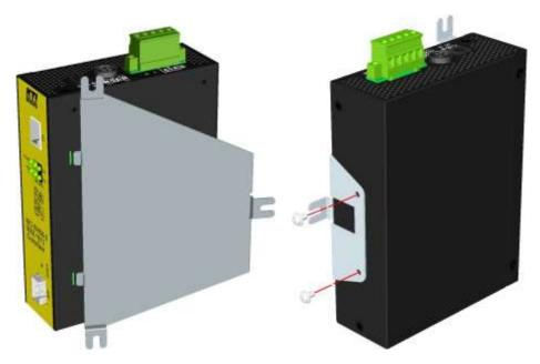
3. Screw the device on a panel and the locations for screws are shown below:
