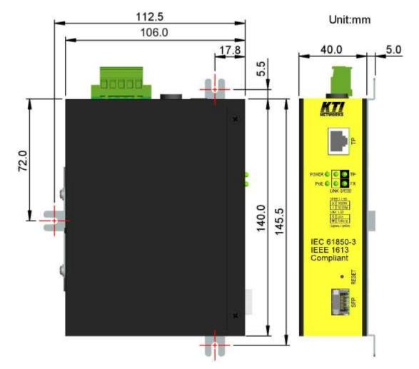
Both models are with same dimension. The final dimension after the bracket is installed is:
