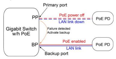
*Note: PoE function on the primary port is kept enabled although a PoE failure is detected by the system.*
