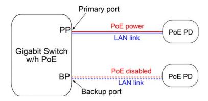
Note: A backup port is disabled for its PoE function and port function by the system as it is configured being a PoE backup port.
