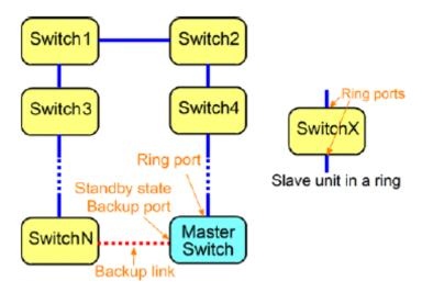
**Slave Units**: All switch units except the master switch in a ring configuration.
