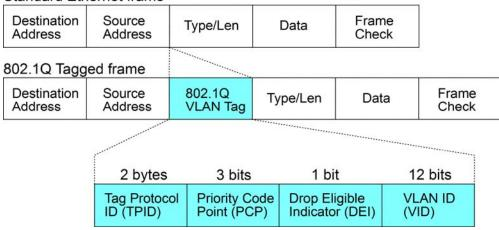
**IEEE 802.1Q VLAN Tag**: In IEEE 802.1Q packet format, 4-byte tag field is inserted in the original Ethernet frame between the Source Address and Type/Length fields. Two bytes are used for the tag protocol identifier (TPID), the other two bytes for tag control information (TCI). The TCI field is further divided into PCP, DEI, and VID.
