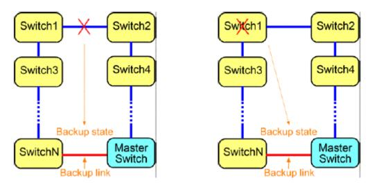
From standby state, the backup link enters into backup state. Other possible faults could be a switch failed due to function failure or power problem as shown in the above right figure.
