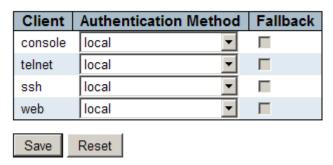
This page allows you to configure how a user is authenticated when he logs into the switch via one of the management client interfaces.
